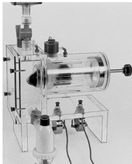
**Fig. 1:** Double chamber bodyplethysmograph (type 855, Hugo Sachs Elektronik, Germany) which is used in our department for induction of cough by administration of tussive aerosols into the front chamber of the plethysmograph.
